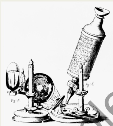
FIGURE 2.1.25 Robert Hooke's drawing of his light microscope in Micrographia , published in 1665
